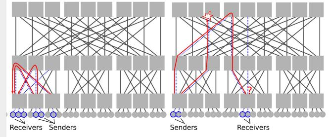
**High Utilization**: This generally helps in reducing fragmentation of nodes and links. The challenge is to provide high utilization while maintaining the isolation and full bandwidth constraints.
