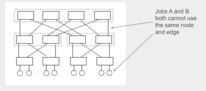
**Full interconnect bandwidth**: ensures that an allocated partition has the bandwidth properties of the fat-tree itself
