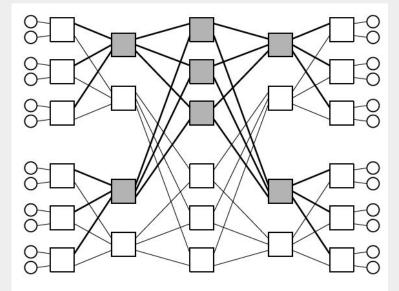
Figure 4: The Clos network equivalent of a three-level fattree. Every node in the fat-tree is duplicated as both an input node (left) and an output node (right), and the tree is "unfolded", sideways, to form a Clos network.
