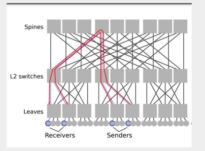
2. Cannot allow full generality in node-to-job assignment. Two flows are forced to share the left-most link in the example
