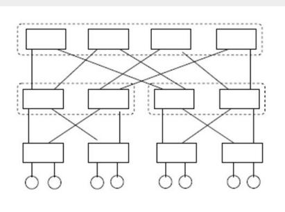
**Isolation**: ensures that jobs do not interfere with each other on the network. This requires that each node and each link be (exclusively) assigned to at most one job. Most existing job schedulers ensure only node isolation.
